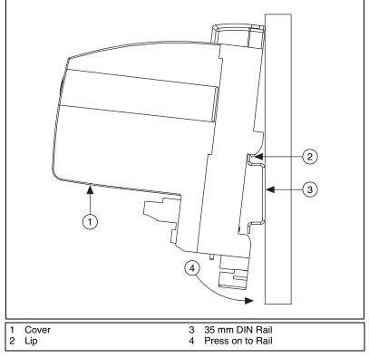
Figure 2-2. Mounting the FBUS-HSE/H1 LD on a DIN Rail
